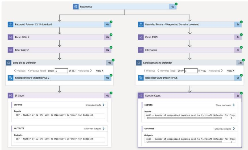
The integration uses a Microsoft Sentinel logic app to deliver high confidence indicators to Microsoft Defender for Endpoint, via the Microsoft Graph Security.
